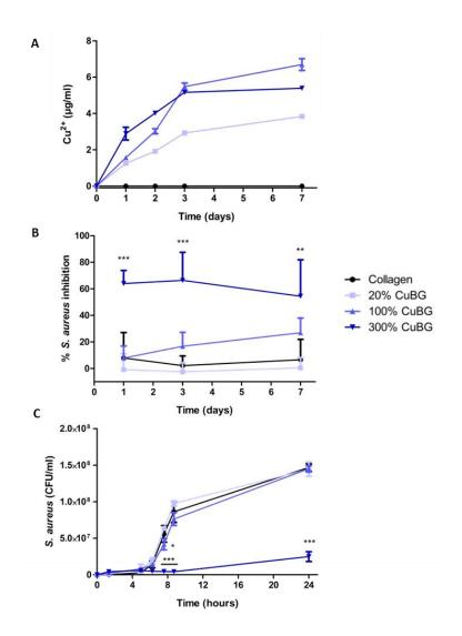
Figure 5 Effect of bioactive glass addition on scaffold antibacterial activity
