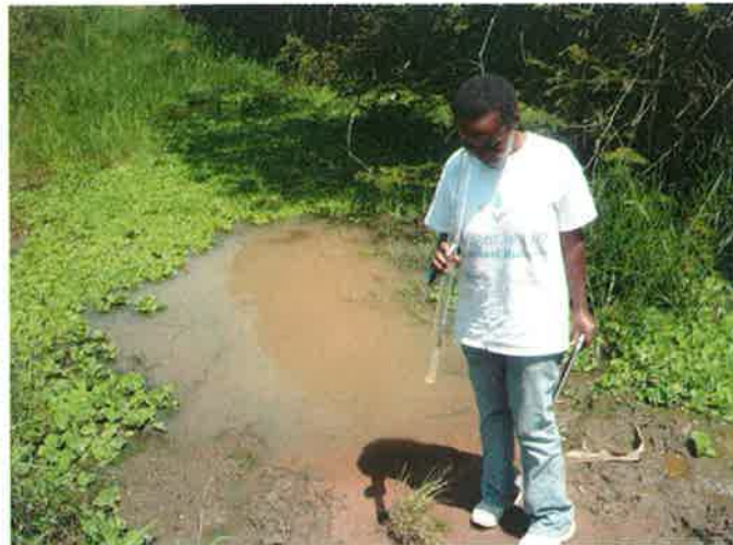
Figure 2.8: Measuring turbidity at an open dug well (Bunjako Primary school)
