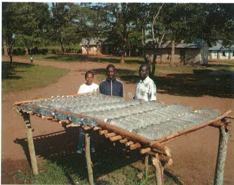
Figure 2.5 : SODIS water treatment on a stand at Misenyi Primary School
